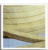
Braided from high quality aramide fibres with PTFE-Impregnation and lubricant additive. Extremely hard wearing. It shows good chemical resistance, high elasticity and very low cold flow. It is wear resistant but may damage the shaft if not used properly. A minimum shaft hardness of 60HRC is therefore recommended. Compared with other kinds of packing, it can resist more severe media and higher pressure. The packing is also lubricated with a silicone-based compound for quick and easy break-in.
