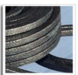
Made of expanded flexible graphite, which are reinforced by textile fibers, with PTFE impregnation. Compared to traditional graphite packing, it has excellent cross-section tightness, structural strength and very low friction-value, wear resistant, yet gentle to shaft and stem.
